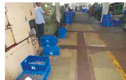
Material lying in Gangway
