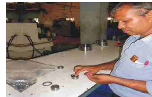
Manual Roller Filling in Cage filling
